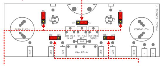
INPUT CAPACITORS CAN BE BYPASSED PER YOUR PREFERENCE. WITH INPUT CAPS BYPASSED, YOU MAY HEAR A SCRATCHY SOUND WHEN ADJUSTING VOLUME. THIS WILL NOT DAMAGED YOUR HEADPHONES OR YOUR AMPLIFIER
